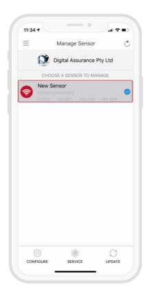
When the Module information is saved successfully to Credential Manager and assigned to the Identity System, the new description will appear in the Manage Sensor tab with a unique serial number assigned.
