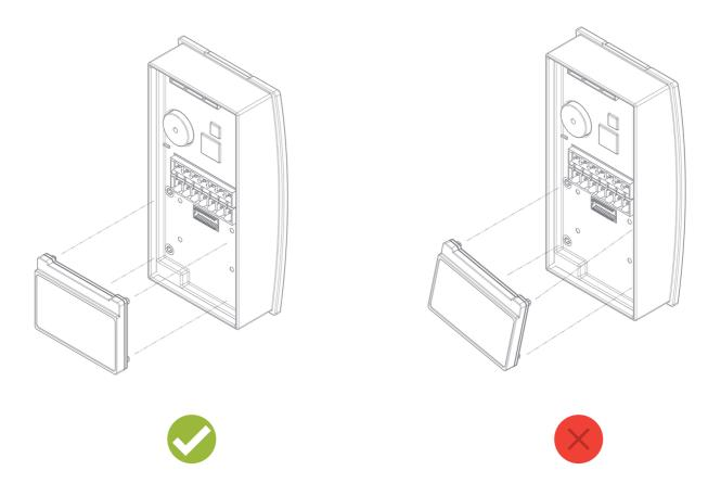
**IMPORTANT!** Installing the SABRE Module incorrectly will cause the PINS in the back of the Module to bend, rendering it as damaged. Please ensure that you position the Module perfectly level to prevent any accidental damage to the device.
