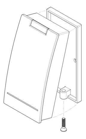
Remove the mounting screw and pull the reader in an 'out and upward' motion to remove it from the wall mount bracket.
