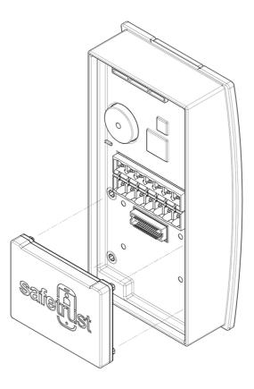
Position the SABRE MODULE onto the reader's connector and press firmly to make a solid connection. The reader's connector is below the wiring — pictured above as a terminal strip however the wiring may alternatively be pigtail.
